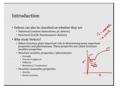
However, if you were to have a copper material without any defect do you know how much can you expect how much is strength should be? It would be of the order of 10 Giga Pascal. So, that is the kind of difference defects make; so sometimes defect can be useful for you, sometimes defects can be bad for you. So, just imagine a world where we had materials without any dislocations and we would have very very high strength material.
