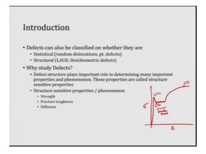
In the previous slide, we classify defects on the base on the basis of dimensions, but they can also be can be classified on whether they are statistical; something like random they have to be there just because of for example, point defects they are thermodynamically stable, structure. So, they will be present at a particular temperature in certain quantity; so they will be statistical defects
