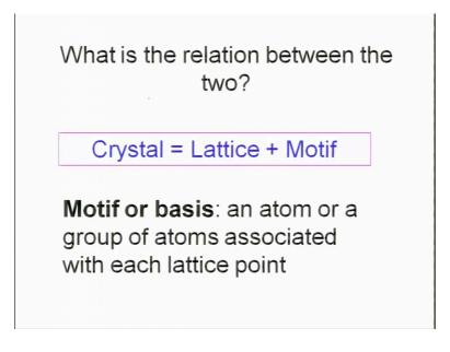
So, basically, we said that the Motif for basis is an atom or a group of atoms which is associated with each lattice point. And I gave you a demonstration of when you put a when the atom is replaced by a molecule that things could be quite different. The definition of primitive a non-primitive unit cell does not remain the same.
