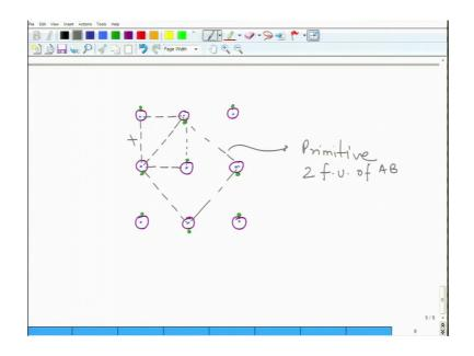
And I put the green atom one here, one there, one here ok. And then one here, one there, one there, one there and one here. So, which is the repeatable unit cell now. Is this the repeatable unit cell? Yes, this is not, right? What about this? So, this is not . So, you will know the straightness, it is not very straight here, what about this? It is so now, this is the smallest unit cell. So, this is the smallest unit cell which means this is the primitive lattice.
