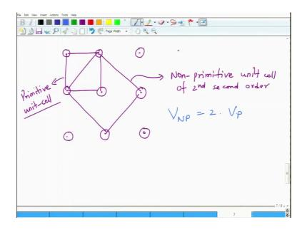
I just draw few of them ok. So, when I said, I have one atom of this, this is one, this is one, this is one, this is one. If I have this off same kind, then I draw a unit cell, this is a repeatable unit cell. This unit cell is the smallest unit cell and how many a atoms it consists of it consists of only one atom. So, this is called as a primitive unit cell.
