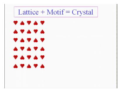
So, this is the illustration of how you can have a primitive lattice with different arrangement of now you can see that each of the heart is arranged in such a fashion. So, that each alternative heart is in same orientation. So, as a result what you have is when you now represent it using the lattice now the Motif is this. So, as a result the periodic lattice does not remain the same as what you had earlier, you need to define it differently.
