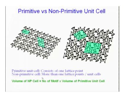
So, I was talking about primitive and non-primitive unit cell. So, basically this is what is the definition of primitive unit cell, primitive unit cell consists of one lattice point. Technically speaking, each atom in this case each animal is a lattice point ok.
