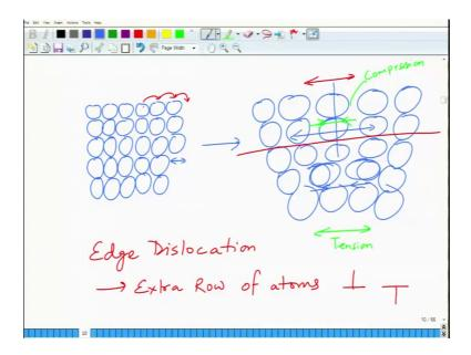
Edge dislocation essentially is an extra row of atoms in the material. So, you have a structure like this which is the perfect structure ok. Now, what we do here is we remove
