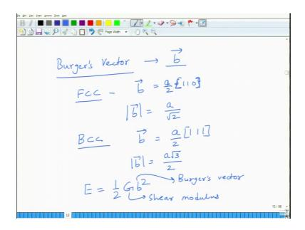
So, for example, in an FCC material b is equal to half of 110 or you can say half of 110 type of direction; a by 2 110. So, the length of b would be equal to a divided by root 2. For a FCC, for a BCC material it would be a divided by a 111 divided by 2 ok. So, this would be equal to a root 3 divided by 2 ok. So, this is how you calculate the Burger's vector lengths that these dislocations have energy as well.
