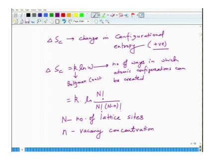
So, this delta S c is basically change in the entropy and this is basically positive in nature as we will see. So, delta S c is equal to small k ln w; where k is the Boltzmann constant and w is the number of ways in which atoms can now be arranged ok.
