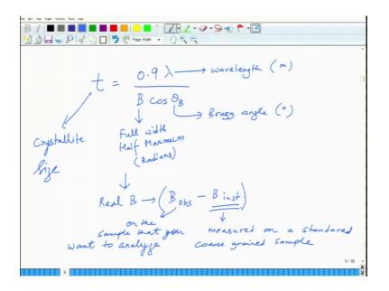
This is characterized by a relation called as the crystal size t is characterized by 0.9 lambda divided by B cos theta B, where lambda is the wave length, B is the full width half maximum which is in radians, and theta B is the Bragg angle in degrees, and this is your wavelength in you can say meters or whatever nanometer. So, this will give you that t which is called as crystallite size.
