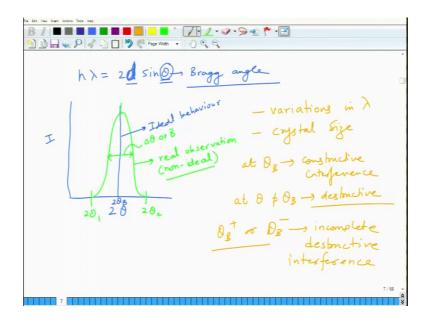
So, ideality requires n lambda is equal to 2 d sin theta which means we must have the value at fixed theta, ok. So, the ideal crystal if you plot intensity for a given peak as a function of, so this is i, this is 2 theta. For an ideal crystal I must have a single peak, a very sharp line because this angle is fixed, ok.
