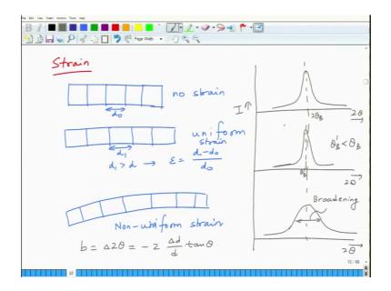
Second thing what you can do is that the strain that is when you have second thing which X-ray diffraction can give you is about the strain. So, this is about the previous thing was about the particle size. You can say particle size or you can say crystallite size. It can give you also an idea about the strain.
