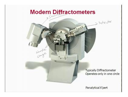
So, your modern X-ray diffractometers look like this. So, this is for example, a panalytical X-ray diffractometer where this is a sample holder. So, let me just use a pen. So, this is the sample stage, this is the source and this is detector. So, your beam, so in this case what might be happening is that your beam may be coming at a fixed angle and this might be rotating and this might be rotating, ok.
