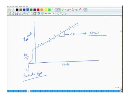
So, what I do now is that I plot basically, so this is a simple linear equation. I plot essentially beta h net cos theta as a function of sin theta. What I can do here is, I can just take this on this side. So, this will become beta observed plus beta. So, this is, sorry this is beta observed, this is beta net plus beta instrument into cos theta, right.
