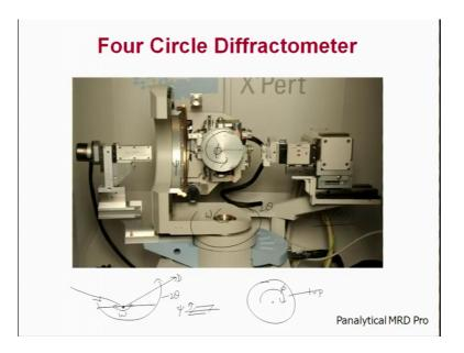
You have a diffractometer like this which has four circle diffractometers. So, you have sample rotating within, this plane you have the cradle rotating within. So, this is phi, this is psi and then, your machine can 2 theta rotates in this and this is 2 theta and then, your sample and then, the sample itself can rotate within this plane. So, this is 2 theta plane. Sample can also rotate along its own axis where, so this is omega.
