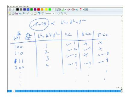
So, this will allow the diffraction will occur and if hkl are mixed, no diffraction will occur, and we did a simple analysis as well where we took a table of thetas. So, we took a table of Bragg angles which we converted into sin square thetas and those sin square theta were converted because we know that sin square theta is proportional to h square plus k square plus l square as a result and h square plus h square h square plus k square plus l square must be integer, right.
