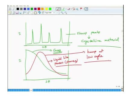
So, when you have X-ray diffraction pattern from different materials, if you plot you will see intensity to theta crystalline material will give you a structure like this, very sharp peaks. So, sharp peaks will mean crystalline material, and the peak width will give you the differences in the grain size and so on and so forth. If you have a pattern like this in which you have I versus 2 theta, you have very broad hump like that.
