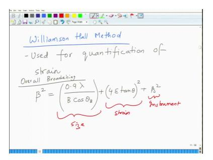
So, this is the strain determination that you can do for quantification of strain. You need to use what we call as Williamson Hall method used for quantification of strain and also, since non uniform strain leads to broadening particle size effect also leads to broadening. You need to distinguish between the two, ok. So, it turns out the overall broadening beta is square.
