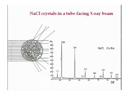
So, this is for example, for a sodium chloride crystals in which face. So, this is in a tube sodium chloride salt powder exposed to X-rays which are emitting in various directions and diffracted x-rays. And what you get a pattern like this. So, you have on the y-axis intensity and this is because X-ray is a photon right.
