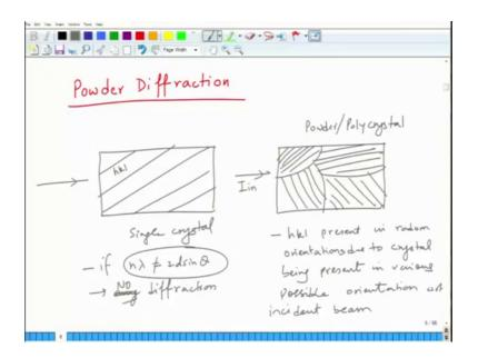
The more common method that we use generally as a material scientist is powder diffraction. And we use powder diffraction because as against single crystal we have plain orientation, there is only one set of plane at given angle with respect to the incident beam. In powder diffraction since the powder, powder is nothing, but multiple single crystals in random orientations.
