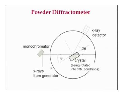
This is your X-rays they go through a monochromator, monochromator or filter. Monochromator only allows the one particular wavelength to be and to go into the crystal this is your sample. So, in this case, if this is your X-ray detector, this is your mono X-ray generator you can rotate the crystal.
