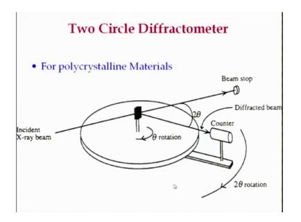
So, this is sort of a modern diffractometer that we will have. So, you have a two circle diffractometer. This is the incident beam. This is your sample. This is the beam stopper for the transmitted beam. You can so this is your incident beam the diffracted beam is going to go in this direction let us say ok. So, instead of putting a photographic film you have a counter. So, this could be a scintillation counter or some sort of detector ok. So, so
