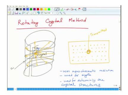
Second method that we talk about is rotating crystal method. In this method, what basically you have you have a crystal ok, the beam hits somewhere like this. This is your crystal. This is your eye in. And you are going to have diffract diffraction going on in various and it is rotating ok, it is rotating.
