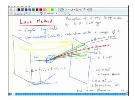
Now, let us look at the various methods, which are used for carrying out X-ray diffraction on various materials. So, we first begin with Laue method which is a method typically for single crystals. And we use basically continuous radiation or you can say white radiation with a range of lambda ok. So, basically what happens is that you have a you have a crystal like this, and this is this is a single crystal in fixed orientation all right. So, this is let us say a single crystal like this ok.
