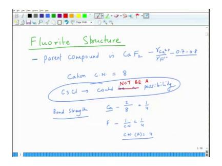
So, basically so the fluoride structure basically is based on compound. So, parent compound is compound is Ca f 2, now this is based on your radius ratio. So, here basically r Ca to r F is such that you tend to follow. So, this is close to I think it is between 0.7 to 0.8 depending upon the radius, but I think it is about 0.8 closer to 0.8 nevertheless it falls in the boundary of octahedral two cubic coordination.
