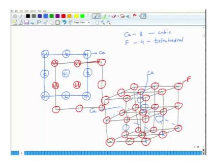
So, if you make a you make it FCC lattice off. So, I am just going to draw the top view here. So, if I draw the top view, so remember coordination numbers calcium is no, calcium coordination number is.
