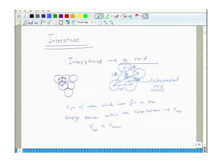
So now, we will talk about new topic in this metallic materials which is essentially Inter stices. Interstices is basically an Interstice is in is a void ok. We can see that, since atoms are spherical in nature, they do not completely they do fill their space but there are voids which are empty ah, there are empty spaces within the lattice.
