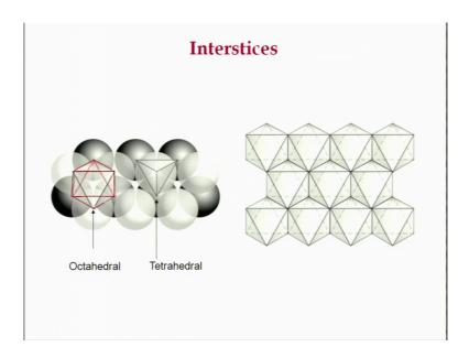
So, this is how the octahedral void looks like in FCC. So, this is the bottom one is the first layer, the lighter one is the second layer the top layer. So, you can see 3 atoms at the bottom; 3 atoms on the top between them there is octahedral void. So, this octahedra is a bit tilted octahedra.
