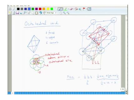
So, here in this case, you can see that this has 6 edges and 4 faces. In case of octahedral, oh octahedral is a body like that. Connect an edge, edge here, you connect edge there, you can edge here, you connect edge there, it has apex here. So, it has 8 faces and 12 edges and 6 corners.
