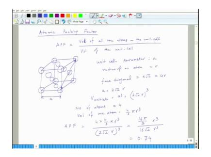
What is atomic packing factor which is A P F is basically volume of all the atoms in the unit cell divided by volume of the unit cell. So, let us say let us see in case of FCC, in case of FCC you have situation like this. So, I will not draw the atoms touching with each other, but they do touch each other for the sake of illustration. So, this is the scenario you have all right now what is so in case of FCC.
