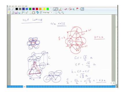
There is something called as c by a ratio, now in case of a hexagonal closed packed we know that there is a and the next set of atoms goes one goes here another goes here and another goes here this is the b layer and the another next layer will again be it will be this layer and slightly displacing it. So, that it is clearer to you it will be this layer, it will be this layer, this layer and it will be this layer.
