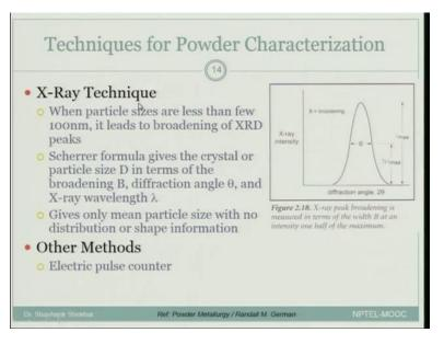
So now let's look at a quickly some one more techniques which is commonly used for determining the particle size and this one is x ray technique. Now when x ray, it is well known that point when you are trying to do diffraction. When you are, when you bombard the particles or the material with x ray, then the materials diffracts and you get somewhere a peak maxima because of constructive interference and at that particular point you have the relation and lambda equal to 2D sin theta.
