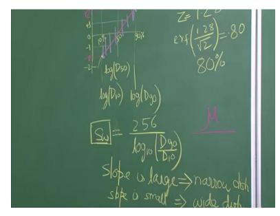
So now what we are saying is that this is the mean so this is D50. So this is corresponding to D50 actually log D50 to be precise. And like I said somewhere over here, you have a 90% data. So this was a 50% data for that matter. And therefore corresponding to that you have log D90. And somewhere over here you have 10% data therefore corresponding to that you have a diameter D10, log D10. And in between this so over here we have we can call it is standard deviation zero.
