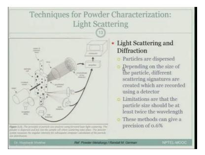
Now similarly there are some more sophisticated techniques, one of them is what is described here. It is a light scattering and diffraction technique. So here is a cell into which you allow the particle to move or feed the particle along which some fluid. Now depending on the particle size and particle point morphology there will be different amount of scattering. And that scattering is captured by a photo diode array over here and some more side detectors that you see over here.
