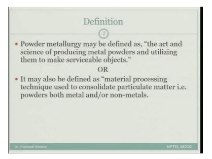
So, let us start with definition for powder metallurgy is the more common term although we are using powder processing because powder processing is for both metals and as well as ceramics. Powder metallurgy since like the term limited to metals or alloys. So, powder metallurgy is usually defined as the art and science are producing metal part powders and utilizing them to make serviceable objects.
