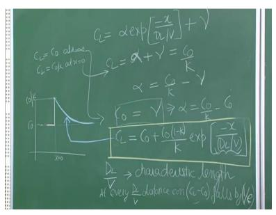
On the other hand, here we are talking only about the liquid concentration, because the solid concentration in the steady state is equal to C0 throughout, in the steady state only in the steady state region. So these are the two different conditions, steady state and the transient state, for the
