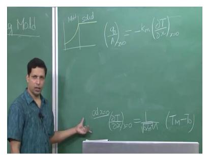
Okay so let us get back to the equation that we left with in the (last) previous lecture; so this is the del T over del x, at x equal to 0, and this is the form of the equation. Now if we want the heat flow rate which is q over A at x equal to 0, that is the heat going in from the solid into the mold, that is what q over A at x equal to 0 means.
