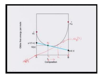
So, lets us now look into this. I just wanted to tell you again that for a system like this, the free energy curve is given by a parabola as a function of composition for a fixed temperature. So, pure ends are given A and B. The chemical potential of pure A is given by mu A superscript zero; chemical potential of pure B is given by mu B superscript zero. But, the chemical potential of a component A or B in this phase alpha, can be measured using a construction known as tangent to curve.
