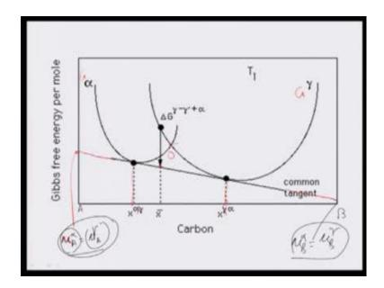
And, find out its equilibrium conditions. So, that is how it is done. Suppose, I have a free energy verses composition curve for two phases of steel; alpha and gamma. Alpha is a BCC solution; gamma is FCC solution. And, it contains carbon as a important solute
