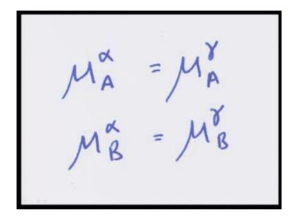
Utility of this is this that we can apply this, this chemical potential equal chemical potential law thermodynamical rule. Rather, mu A alpha equal to mu A gamma mu A beta mu B alpha equal to mu B gamma for a two phase system.
