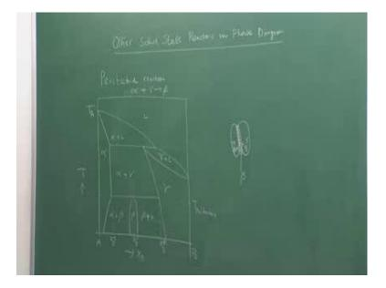
Peritectoid, so this is what is the phase diagram this is temperature axis, this will be the composition axis between two components A B; liquid, alpha, alpha plus liquid, and then this is gamma plus liquid this is gamma alpha plus gamma, beta alpha plus beta, beta plus gamma that is what is a peritectoid reaction thing. But here actually I am showing
