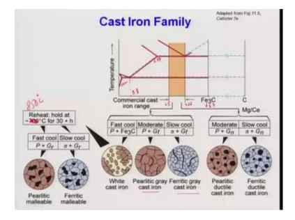
Now, in next 5 to 10 minutes what I am going to do is I am going to discuss with you the in one slide? How things happen as you know, this is the iron carbon phase diagram these are the commercial range and I am just showing you a temperature versus composition. This is the commercial range of the for the cast iron family as you see here.
