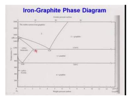
On the other hand this is the graphite phase diagram, you see here this is 2.14 this should be 2.14, 6.8 to 4.26 eutectoid transformation temperature is about 700 and 36, and this temperature is 1,154 degrees Celsius temperature.
