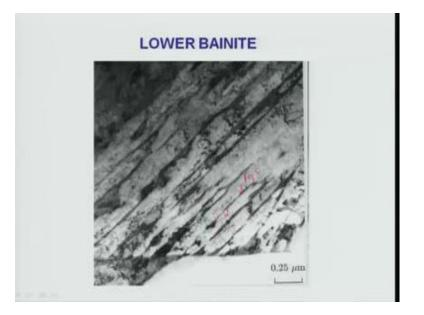
These are the plates of alpha. These are, each one is alpha, and these things, black color thing, are Cementite. So, Cementite is precipitated at the boundaries of alpha, not inside the alpha; that is a distinct difference. In case of upper Bainite, Cementite precipitated
