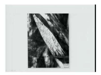
So, as you see here, very clearly, this is the t m picture; as you see here, this is the long sheath of this alpha and inside of this cementide is precipitated out. This is what is your upper; and, lower one will have plates of alpha.
