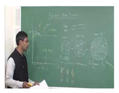
So, now let us go into how many different ways of alpha can form? It seems there are, actually I also forget, so I have written down in the page, there are actually five different, four different phases of alpha. I will write down one by one and let me do that here. So, first one is known as grain boundary alpha, the one I have drawn.
