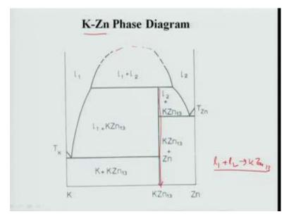
This 1 is a potassium zinc system, which is not at all used in the real applications and you see here this is the dome and then there is a line compound K-Zn 13. It forms by the syntectic reaction K-Zn 13. So, again align compound and these forms this, this we have discussed in the in case of peritectic reactions.
