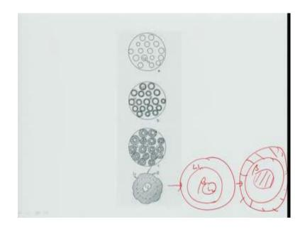
Now, how the things happens in a syntectic reactions. So, before I do that let me go back here and I take this alloy this alloy and I discussed you can see here this alloy and below T c, you will separate into L 1 plus L 2. So, below T c it will have 2 liquids L 1 and L 2 and both of the liquid will have different densities depending on density either L 1 will float or L 2 will float, let us suppose L 2 L 1 floats on L 2. Now, what will happen that
