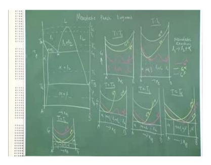
This is for any system A and B as a function of composition temperature. So, this is the melting temperature of pure A, melting temperature of pure B liquid and this is the T c above which single liquid present below, which it separates the 2 liquids alpha plus L 1 alpha plus L 2 and alpha plus beta and this is beta. Now, there is some problem here let me complete it. So, this phase field is beta.
