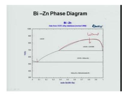
Now, there are some other examples let me show you; like this is again from betas beta this method is zinc, you can see here there is a dome here, and that dome indicates one liquid phase going to liquid two and liquid one and liquid two, and then there is a monotectic reaction here, sorry monotectic reaction there; that becomes liquid plus zinc s c p. So, let here look at micro structure you can use this kind of system to create nano structures.
