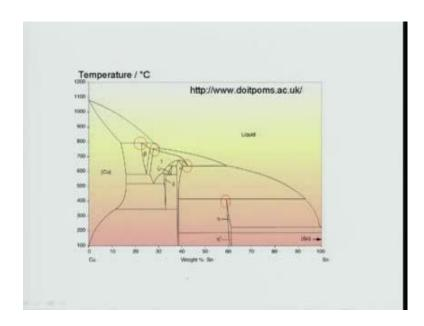
Similarly, for copper tin system which is a basically a bronze, you can have a peritectic reaction; several one; one, two, three, four are shown here at different temperatures. So, beta bronze or epsilon bronze or eta bronze, they are all produced by peritectic reactions, different peritectic reactions. And, just to show you a picture on microstructure of that this is your alpha beta bronze.
