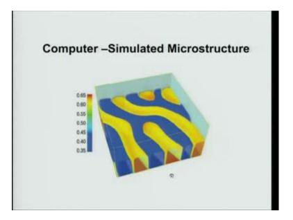
So, this is the green slab or the blue slab, this is the yellow slab. Sorry this is the blue; sorry this is the yellow slab. You can clearly see that they are actually looking like long slabs in three-dimensional and when you cut it using a two-dimensional section, they would look like a lamella.
