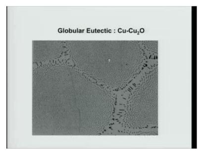
There is another type of microstructure known as globular eutectic. What is that? It is normally found between cu and cu2o. If you have a copper melt and if you have sufficient amount of oxygen present in during certification, then such a kind of things forms here c u o is basically looking like continuous gray color stuff.
