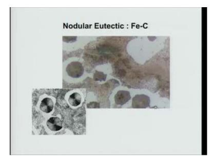
Another classic example of eutectic alloys, irons, carbon or rather cast iron, all are pure. We are in the industry they know the cast iron is the most important material for automobile industries. It has lines see as in automobile industry. So, cast iron has a eutectic phase diagram and eutectic is between gamma iron and carbon or graphite. So, you can see here this is the graphite nodules. They are like the nodule.
