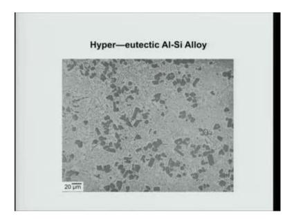
Then you have eutectic in between. So, I will again come back. Another one is hypo eutectic alloy. You will have silicon. No dendroid silicon has a piece. You can see here silicon hesitated silicon crystals around and the eutectic and these silicon crystals are brittle there. So, hyper-eutectic aluminum silicon alloys rarely used in the applications.
