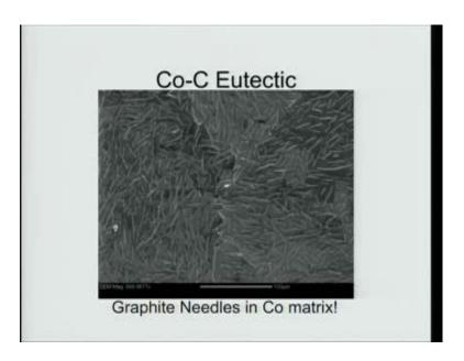
Now, there is another eutectic which is copper eutectic. We see here, here also the carbon copper co by matrix carbon eutectics. Carbon is coming as a graphite needles here and co by matrix is a continuous gray matrix. So, I have written graphite needles in a co by matrix very important material because of strength.
