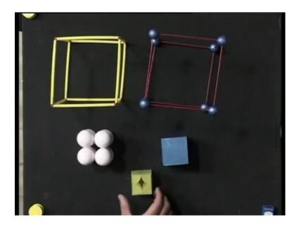
So, I have in front of me an example of the four kinds of models I was just talking about, in addition I have got a fifth kind of the model, which I will talk about. So, the left hand side I have got an yellow wire frame model, this is my ball and stick model, this is my space filling model and here, I have got my void model.
