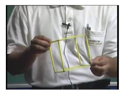
As you can see, in the wire frame model, which I will pick up and show you in perspective, the vertices are the seats of the lattice points and of the spherical atoms. And these wire frame models are important for us to understand the connectivity and also perhaps the unit cell shape. So, here, so this is the first class of models, which I can use and we will see more example of these kind of wire frame model when we go in the course along.
