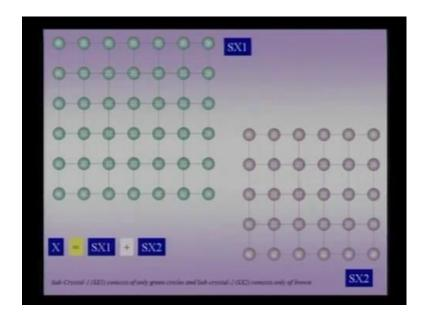
Then, I actually split out this super crystal if you wish to call that into the two sub crystals, the sub crystal 1 and the sub crystal 2. And you can clearly see, the sub crystal 1 is fully decorated with the single circle motif and sub crystal 1 can itself be thought of as an independent crystal, wherein you got a square lattice or in this particular example, a rectangle lattice decorated with a green circle.
