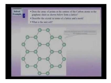
And this is the example a graphene sheet, so I shown here a part of the infinite graphene two dimensional layer. And you can clearly see that, in a graphene sheet, you have carbon atoms which go on to sit at various vertices of this hexagon. So, you have a grapheme sheet which is here and you all know, this graphene sheet is high speed to hybridize and it is, ideally speaking in a more mathematically way, it is actually two dimensional.
