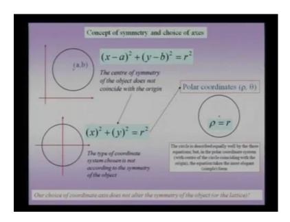
A simple circle described by two Cartesian coordinate system, one is here on the left and one below that and one polar coordinate system. Now, the equation of a circle, suppose I want to describe the circle in terms of this left hand or the Cartesian system given in the left hand side of the slide is x minus a the whole square plus y minus b the whole square is equal to r square. Now, let me now move the circle to the origin, which is the (0,0) point in the coordinate system.
