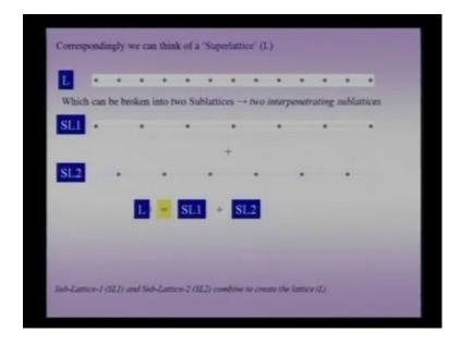
So, let us now talk about the sub lattices, which go on to make this sub crystals and the crystal itself. Now, suppose, I consider this array of points, over which this arrows, up and down arrow were sitting, this itself can be considered as a lattice. Once I decorate this lattice with up and down arrows I clearly see that, the blue dot or the set of blue points no longer remains the lattice point. But, if I just consider the array in independence then, I can always think of this as lattice.
