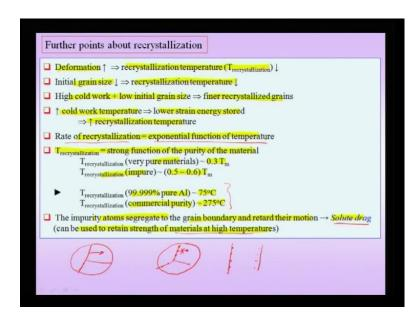
Now, if this re-crystallization or the working itself is done at a higher temperature, wherein re-crystallization can take place, actively during working such are re-crystallization would actually be called dynamic re-crystallization. That means, that I do not have to have a separate re-crystallization step between the working steps therefore, I am doing working at hot working. And again let me one once more that these term terms like hot working, and cold working are technical terms.
