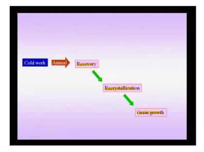
Now, therefore, during annealing you can and if you give a sufficient kinetic energy, suppose you are holding at high temperatures. You would have recovery followed by recrystallization followed by grain growth, in the case of even high temperatures there would be recovery. But, then since the dominant process re-crystallization we have written it as re-crystallization, so in the whole process we will see that the physical properties of the material changes.
