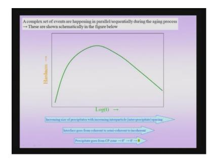
But we go through a complex sequence of precipitation which involves intermediate meta-stable phases like theta double prime and theta prime.
