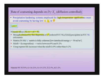
We can either use a precipitate which has a low gamma. That means that the 3 strategies which we can use avoid the coarsening of the precipitate which is especially true if your alloy is used at in high temperature applications where the coarsening chances are very large. Then we can use either a low interfacial energy between the precipitate and the matrix to reduce the coarsening rate. We can use a an alloy for which the diffusivity is
