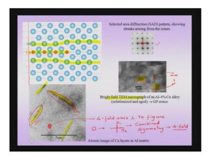
So, you can see here suppose I consider this the half picture of the GP zone that means that the GP zone itself extends the other way about this is a mirror plain mid plain. And this is my disc of copper atoms right in the middle here. And this is what we call the GP zone and this is the copper red zone. And as I said it can be thought of a speakers to a precipitate and if you look at the area present in the matrix this thin copper layer which we pointed out can be about 2 atomic layers thick.
