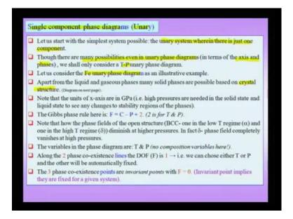
The unary system is such a system, in which there is just one component, in other words composition cannot be a variable in a unary phase diagram. But, still there are many possibilities, even in unary phase diagram in terms of the axis and the phases, which form. For an illustrative example, let us consider the iron unary phase diagram, in which we have temperature and pressure acts the variables, the thermodynamic variables which are varying.
