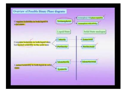
So, we will consider an overview of possible, binary phase diagrams based on the solubility criteria. So, the complete the first case is of course, there is complete solubility both in liquid and solid states and these are called isomorphous phase diagrams. And even within isomorphous phase diagrams, there are cases where even though there is solid solubility.
