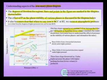
So, let us dwell a little more and try to understand, some of the points we already make and try to introduce, some more concepts in understanding of the iron unary phase diagram. The degrees of freedom for regions lines and points, in the figures are marked in the diagram as shown before, so these are the various regions in the phase diagram, the effect of pressure on the phase stability is also discussed in the diagram below.
