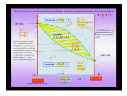
So, let us go ahead and map the degrees of freedom in various regions of the isomorphous phase diagram. So, in the binary phase diagram we have of course, the two pure components, which is a on the left hand side and b on the right hand side for the pure components. Of course, C is equal to 1 and therefore, you can write down the phase rule as two minus P.
