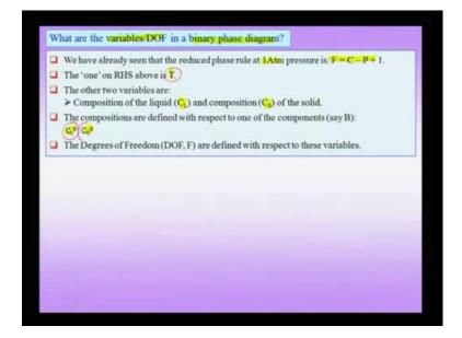
So, before we proceed further we have seen that, when we talked about the unary phase diagram the only variables possible where pressure and temperature. And there were no further variables to be considered. Because, the component was just one and therefore, there was no need to talk about composition variables, but in a binary phase diagram, we need to understand, what are the variables and degree.
