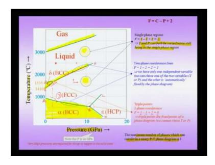
And so, let us have a peak into what the unary phase diagram we talking about, so we are talking about a unary phase diagram of iron, where pressure is one of the variables along the X axis and temperature is the other variable along the Y axis. Therefore, there is just one component, which is iron and we are varying these two variables to find out, what happens to the phases as we change the temperature and pressure.
