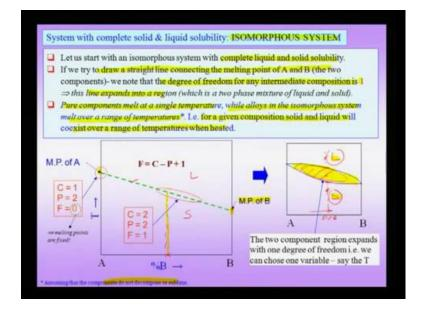
So, let us start my understanding what are isomorphous phase diagrams or an isomorphous system, as we have pointed out an isomorphous system is one where in
