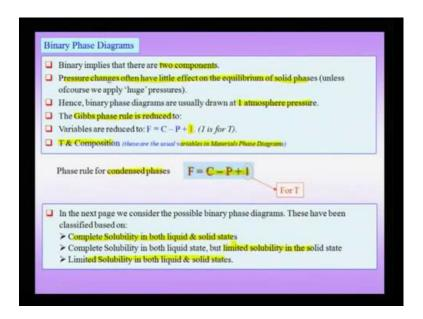
Now, let us proceed further and try to understand what are called binary phase diagrams, the fact that the word binary is used implies, that there are two components. And these two components, as we have already noted can be elements like copper and nickel, they could be even compounds like alumina and chromium. So, we will take up some examples to understand these kind of phase diagrams and we have already noted that pressure changes, often have very little effect on the equilibrium of phases.
