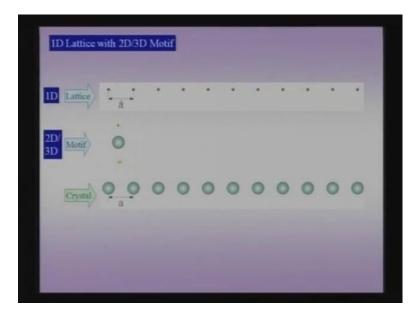
So, let us start with the lattice which are one dimensional lattice before with a lattice parameter a. Of course, I can put a spear or a circle as a motif in each lattice point and therefore, I can get a crystal as in a figure below, which consists of a periodic arrangement of circles as spears on a one dimensional lattice.
