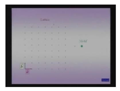
As in the case of one dimensional crystal, a two dimensional crystal is nothing but a two dimensional lattice, which has been decorated with a two dimensional motif. And as before we can actually relax this requirement, by putting one dimensional or three dimensional motifs on to a two dimensional lattice, to generate a crystal which is not actually truly two dimensional, but has a dimensionality between that of a lattice and motif.
