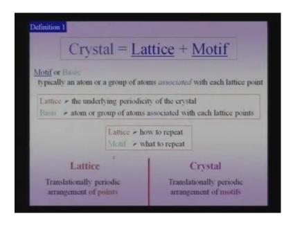
So, what is a lattice? At the first look we can understand the lattice to be the underlying periodicity in a crystal. So, a lattice actually captures underline periodicity of a crystal, a basis actually is any entity typically as we shall see, it consists of an atom or a group of an atoms associated with each lattice point. We will take up examples these to clarify the points, but the key word when we are talking about basis, the word associated which been highlighted.
