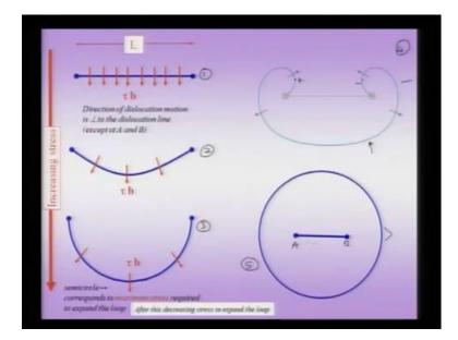
Now, suppose I keep increasing the stress, then what would happen is that the dislocation line would bow more and more, this segment which is unpinned, the segment which is free to move, would in an increasing stress lead to larger larger bowing. The upper limit for this radius would be the radius, where in this becomes semi circle and entire process starting from figure. For instance, this point 1 to 2 to 3 will take place appealing stress,
