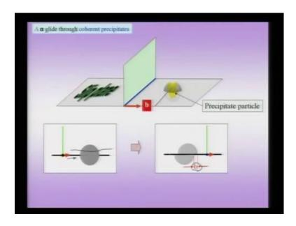
Now, suppose I have a precipitate line on this slip plane, and now this is a coherent precipitate right here, sitting on the slip plane, and now I have dislocation line which is shown in blue moving on this slip plane, try coming to this precipitate. Now, I can actually see this precipitate on the side view, where in I have dislocation line here, and the dislocation is moving towards may right into the grey color precipitate.
