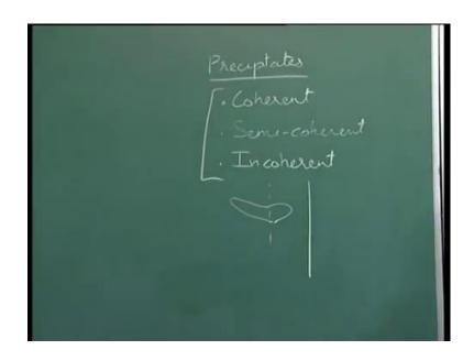
So, here three types of precipitates out here, and the coherent precipitate is a precipitate in which the atomic planes are continuous from the matrix into the precipitates, in a semi coherent precipitate there are regions in which the atomic planes are continuance. And there are regions with atomic planes ends at the interface, and that they can be interpreted as the presence of an dislocation.
