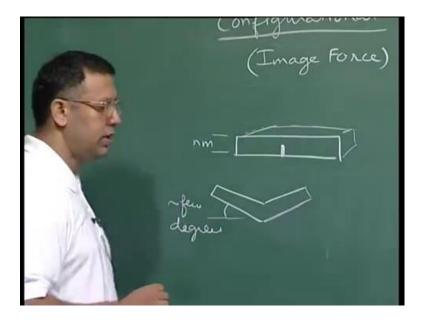
But, you have to remember now, this bending is a coming, because now introducing at dislocation into a flat place, which originally was completely defect. So, you can have what you might call deformation of this type, which are purely elastic deformation coming from the presence of dislocation, so this is something which again is important to noted.
