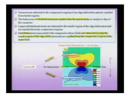
Now, let us start with an interaction of vacancies with the stress field of the edge dislocation, so in the figure below you can see that, actually I am showing the sigma x stress field around an edge dislocation, that dislocation line is into the plane other board right of the center here. And so, let me mark that, so this my edge location is right of the center, and you can see that the entire half space about is tensile in nature, and entire half space below is compressive in nature.
