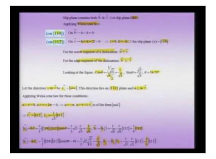
Now, if the direction perpendicular to t is t perpendicular is u v w, this directions lies on 1 1 bar 0 planes the slip planes, and this perpendicular to the t vector, so this is obvious. Now, I can again apply ways on law assuming this 2 conditions, for the u v w direction, which is now the directions perpendicular to the t, and this for applying this on this 1 1 bar 0, u = 0.
