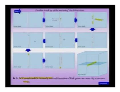
So, how is the kink pair operate, suppose I had perfect dislocation line, I can have a king the dislocation line, and I am not talking about the double kinks, and as I show slide here that these kink scan be created by thermal fluctuations. So, thermally activated you can have a double kinks formation, and I pointed out what is the kink, a kink is a defect in a effects, dislocation is a line defect in the crystal a kinks is a defect in the dislocation line.
