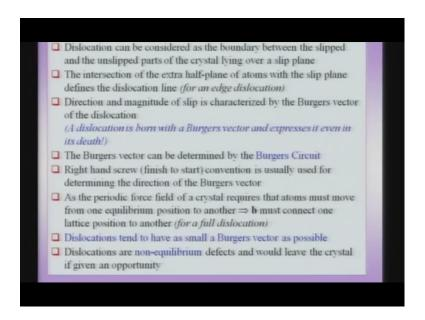
So let us summarize some more important things. We consider so far with regard to dislocation stage especially a dislocation can be thought of as the boundary between the slipped and the unslipped parts of a crystal line over the slip plane. So, again as I told you this is just a way of visualizing the edge dislocation and often it may differ dislocation exists in a crystal. it may you cannot tell which is the slip part or which is the
