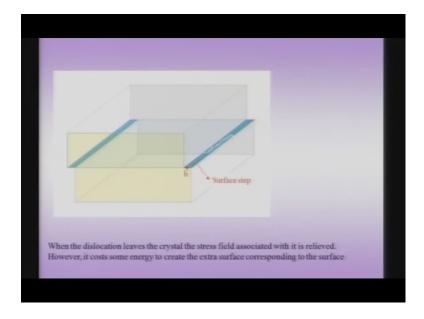
So this is my surface step which has been created by the motion of the screw dislocation. And as before all these stresses associated with the screw dislocation are relieved and, but a small energy is added to the formation of this extra step which is now I surfaced.
