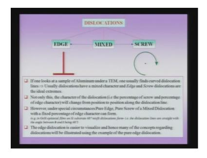
Now, it if I look at a sample of aluminium under a TEM, it pointed out typically one finds a curve dislocation point. That means there is lot of dislocations typically simple sample of aluminium, even it is a well unyielding sample. You will find lot of dislocations in a transmission electron microscope, and when you if you take a deform specimen like a deform specimen of aluminium which is been may be deformed in anyway.
