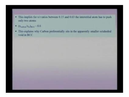
To summarize, this x by r ratios between 0.15 and 0.63 and again pointing out this are some so on. So, the simplified calculation the interstitial atom has only push two atoms and therefore, it would go and sit in any octahedral void. So, with we have made a sort of an overview of all the void which are present in the cubic close pack crystal the body centered cubic crystal and the external force pack crystal.
