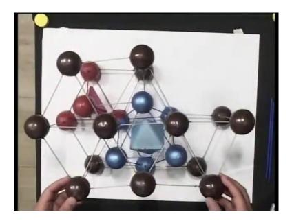
I have here a model of the external close pack crystal wherein I have three layer of atom. The Bessel layer, there is one layer of atom in the middle which is pointed out, goes part of motive and there is a third layer above. Here, I want to illustrate the presence of the octahedral and the tetrahedral voids. Let me start the easier of the two which is the tetrahedral void and as a point out the tetrahedral void is made by the atom in the Bessel plane and an atom which is sitting above.
