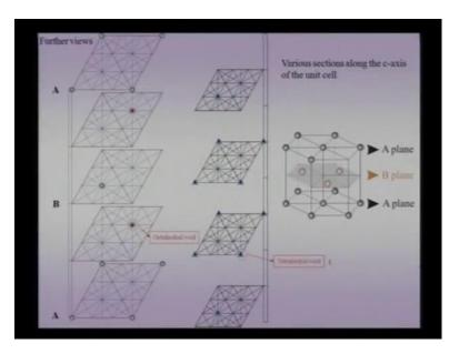
Wherein the hexagonal unit cell has been spit into various planes, so this is plane for instant located at 0, this a plane located at half, this is a plane located one-fourth, this is three-fourth and 1. Similarly, there is a diagram right hand side which is been you stood locate the position of the tetrahedral void. So, you can see that if you look make such a
