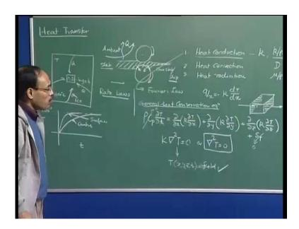
And therefore, what you conclude that well, you know, it is the flow of heat assisted by fluid motion which is the fan, which is flowing the heat into the room is much more rapid than the conduction heat or the radiation heat. Also you can imagine will you have
