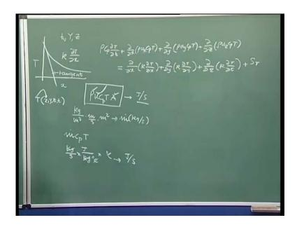
So, we can say that if we take look at this particular term multiplied by area, so, what is rho? rho is kg per meter cube; u is meter per second; area is meter square. So, this term rho, u and A, this basically is nothing but meter cube meter cube cancel, so, this is actually the mass flow rate which is kg per second.
