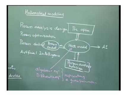
So, this mathematical model that I have here as I mentioned that, it is either an algebraic equation or differential equation representing a given phenomenon. So, unless and until, I say what is that phenomena, we cannot develop the model, we cannot formulate the algebraic equation or the differential equation.
