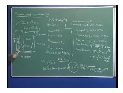
We must understand now. So, geometric features are scaled. So, plug location – two third of R, which is equal to bottom; so, which is 1.233 divided by 2. R is diameter divided by 2. So, this this cancels out. And therefore, this is roughly going to be 0.4 meters. So, that is the plug location in the model itself. From the axis of symmetry, I
