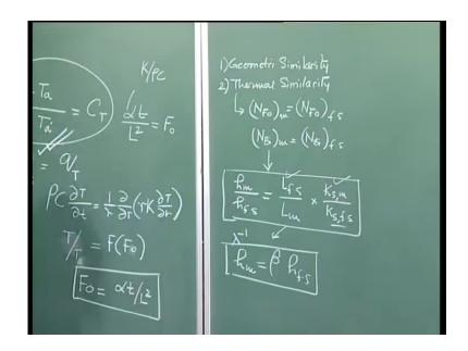
Therefore, this particular expression will give me that look h model is equal to some constant beta into h sub f s in which beta is nothing but lambda inverse multiplied by k s m divided by k s, f s. So, having known the value of heat transfer coefficient in the full scale system, I should be able to adjust my heat transfer coefficient in the system in such a manner that this condition is going to be maintained.
