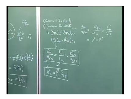
Similarly, the Fourier number equivalence will tell me that look I have t model by t full scale. That is going to be alpha model alpha full scale. So, alpha t and then L square; so, this is going to be L model square by L full scale, which is equal to lambda square into some constant, maybe the biot. Thermal conductivity – this is k divided by rho C. So, these are material-dependent properties; thermal diffusivity.
