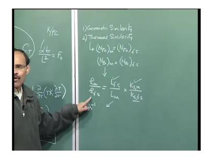
So, I know the ratio of the thermal conductivities of the two solids. If I have the solid, which is steel in full scale system, I know the thermal conductivity of steel. If I have taken copper, I know the thermal conductivity of copper. So, this term is known; this term is known.
