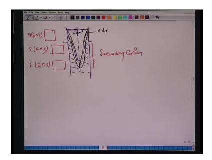
Now, if I want to show here, for example, if I draw very symmetrically, say this is the mold, here there is a partially solidified strand; this is the wall shaped mashie zone. So, here, all liquid; what I wanted to show here is all liquid. This is the mold; this is the solid; this is the solid shell which is growing in it thickness as we move downward the mold and this is here all solid.
