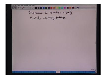
So, what one thing you have to require? You increase in tundish capacity, you increase in tundish capacity. If the tundish of a high speed slab caster has also to remove the inclusions during the process of continuous casting. So, increase in tundish capacity. Well, if you cannot increase the tundish capacity, then what you have to do? You modify steelmaking technology. These are the two solution that are coming in my mind; may be still another solution you can think of and see what can be done.
