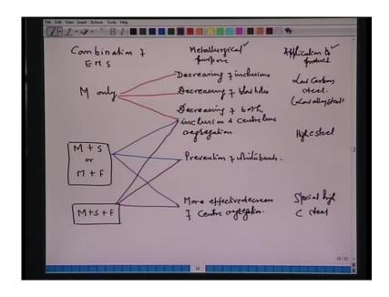
Now, say some of the say combinations of EMS, in some plant, the combination of electromagnetic stirring is done, the metallurgical purpose, metallurgical purpose, and application to product, application to product.
