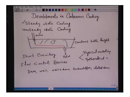
Let me introduce to you now two terminologies - one is the steady state casting, steady state casting, and other is unsteady state casting, unsteady state casting, because as you pour molten steel from ladle to tundish, it takes some time before the tundish attains the required height; between that period, the casting proceeds, and that period is called unsteady state casting, that is, during the unsteady state casting, the molten steel bath height in the tundish change.
