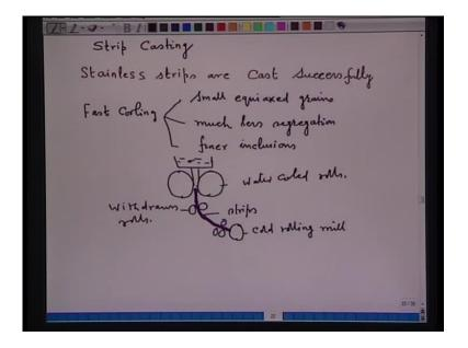
So, at present, stainless steel stripes are cast successfully though attains are also being made to cast carbon steel stripes, carbon steel stripes. Now, as molten steel is cast directly into the strip to the cooling is to be very fast. Now, the fast cooling has some very important features. So, the fast cooling may result in small equiaxed grains, much less segregation.
