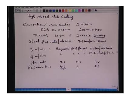
So, I have thought let me take it. Say let us consider a conventional slab caster; say let us consider a conventional slab caster, which is casting at 2 meter per minute. The slab cross section is 280 millimeter thick into 1950 millimeter white. It is casting having a tundish 70 ton capacity and 2 nozzles at the bottom of the tundish; that means 2 strand caster; it is a 2 strand caster. So, if I calculate now a steel flow rate per strand, very
