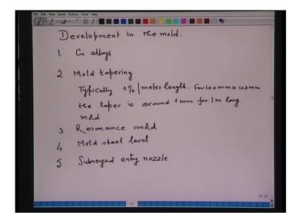
So, the tundish slag is selected such that it has both the roles during the continuous casting. So, this is about the development in the tundish. Now, say development in the mold, development in the mold. As I have said, that mold is again a very important part of the continuous caster; several developments have taken place.
