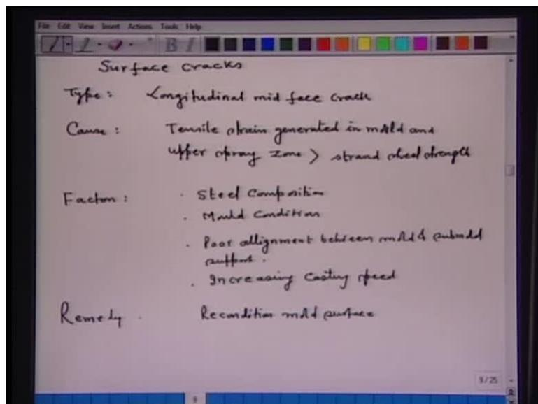
Now, similarly I give a few examples for surface cracks. Surface cracks, the types and remedies. Say, type, take for example, longitudinal mid-face cracks; cause, it can be tensile strain, generated in the mold, and upper spray zone is greater than strand shell strength; that means, when the tensile strain generated in the mold and upper spray zone, when it is greater than the strand shell strength, naturally a surface crack will form. Now,
