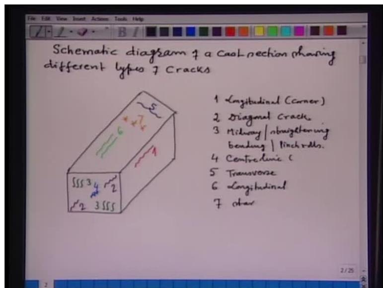
So, what is the origin of cracks? Now, before you go, I would like to show you the schematic diagram of a cross section is showing different types of crack. Now, one is the longitudinal crack, longitudinal corner, which is shown by the red mark. Second is a diagonal crack; third is the midway, or straightening, bending to pinch rolls; then, fourth is a center line crack, which is shown by the blue color; then, fifth is the transverse, and
