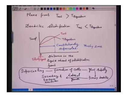
So, it is the movement of solid liquid interface. Now, we can have either a plane front solidification, either a plane front solidification; this plane front solidification can occur, when temperature, the actual temperature is greater than liquidus temperature. Now, this situation can occur, when no segregation is involved; due to segregation of solute, the
