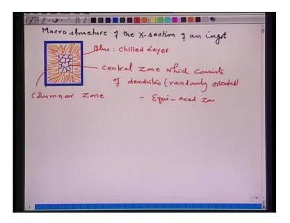
Now, suppose, if we pour a killed steel into the mold. And, you would like to see, how the macro structure is developed in the ingot. So, for that, let us see the macro structure of the cross section of an ingot. So, this is, the blue one, blue color, that is, this one is a chilled layer; mold is water cooled; as you pour the liquid, the liquid which is in contact with the surface of the mold, it gets immediately chilled. So, as such, we have the chilled
