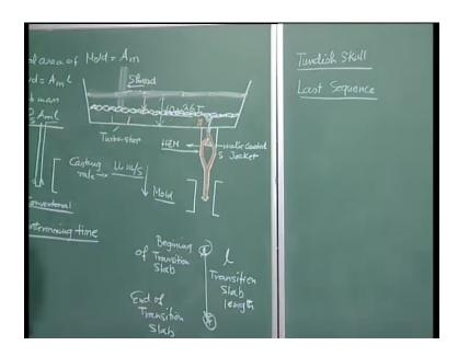
If you do not stop the casting, what happens; slag will be entrained and this slag which are oxides, they are going to make steel weaker and as a result of which we can have innumerable problems, and nobody is going to buy that steel which will contain lot of entrained slag particles itself.
