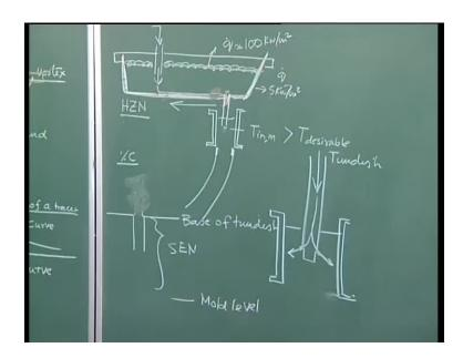
What is the extent of heat loss in Tundish. For example we can have, we look at this figure here and say single strand slab casting Tundish, operated under steady state condition. So, you have a heat flux operating here, which is of the order of 100 kilo watt per meter square, that is the kind of and we are talking about 5 kilo watt per meter square, so which is operating through.
