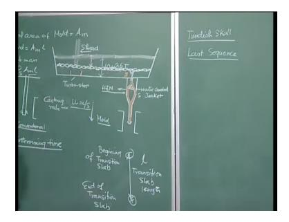
Now, the last topic; last but one that is the Tundish skull, and before we must remember that the casting rates are different for different processes, they depends on the number of strength, they depend on the cross section of the product and so on.
