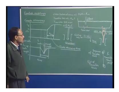
So, this is the time I have brought in a new ladle, and after I open the new ladle, the bath height increases and then I bring it to the original level as is shown here.
