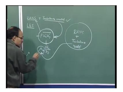
The turbulence model actually provides us the distribution of mu t in the domain through an appropriate mathematical framework. So, we obtain mu t from the turbulence model; we substitute that mu t into the RANS equation, then the RANS equation boils down to four equations, four unknowns and we are in a position to solve and obtain meaningfully the velocity fluid, which are prevalent in steelmaking reactor.
