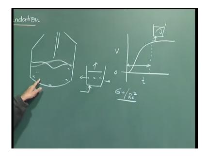
So that looks something like this. So, for example, if you plot velocity at a location versus time with gas injection in a ladle - small little figure I draw, so I introduce a gas here and then, the flow develops and you see the flow goes something like this.
