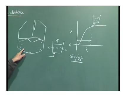
So, it depends on the process in which we are looking at. If you are looking at the initial period of gas injection, the flow is unsteady; if you are looking at a long duration of gas injection, in that case we can say that the flow is steady.
