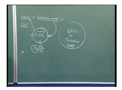
One last point that I want to say that this term -Reynolds stress term- is the essentially formulated in terms of, if you put a minus sign and you can say the turbulence viscosity and the velocity gradient, so we have if this is only in meaningful velocity gradient is this d v x over d y.
