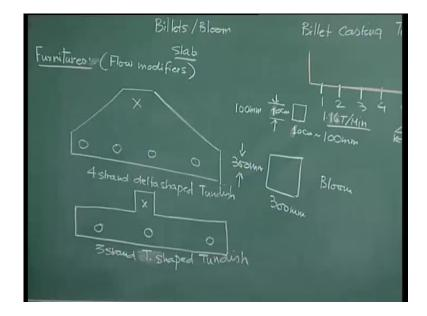
Also I have drawn a tundish which basically looks like a rectangular shaped tundish. If you look at the cross section and the cross section for the top view of the tundish will look something like this. So, it is a rectangular shaped tundish, but it is not necessary that all the tundishes are going to be always rectangular cross section.
