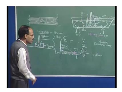
So, the turbo stop, actually the placement of a turbo stop can create surface directed flow. It can prevent also entrainment of the slag, because the flow, you know the upward direction flow here, the flow is moving up; the flow is moving down here. So, the flow can be significantly reduced, and as a result of which, the entrainment of slag can also be or the mixing of the slag or opening of this area can also be substantially eliminated.
