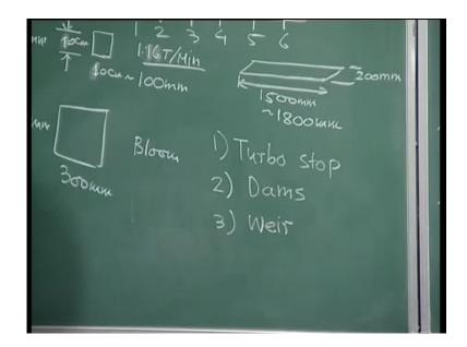
Number 1 is Turbo stop this is common number 2 Dams and number 3. These are the 3 essential or the basic types of furnitures which are normally introduced in the tundish. What is the objective of introducing such furnitures in the tundish?
