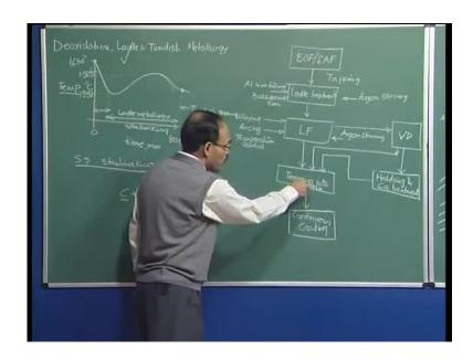
Therefore, this equation which I have written here under reduced carbon monoxide partial pressure or reduced pressure within the system, because whatever carbon monoxide is forming, may be you can draw here a line that through this or suction is going to be applied and all carbon monoxide is going to be taken out, and as a result of which, this is maintained at a very low pressure, and under low pressure, this equation will be driven towards the forward reaction.
