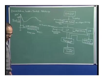
So, first we start with a BOF and an EAF. - Basic Oxygen Furnace or Electric Arc Furnace steelmaking - So, this is the primary steelmaking; followed by that, we have tapping operation, and this is tapping and we have ladle treatment, and basically in this ladle treatment, we are talking about argon stirring, and what we are doing in this ladle following tapping is nothing but deoxidation, may be we are doing aluminum wire feeding or bulk deoxidation.
