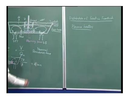
We can now talk about the distribution of temperature a little bit; distribution of heat in tundish. It is often required that if the temperature drop of this material is significant,
