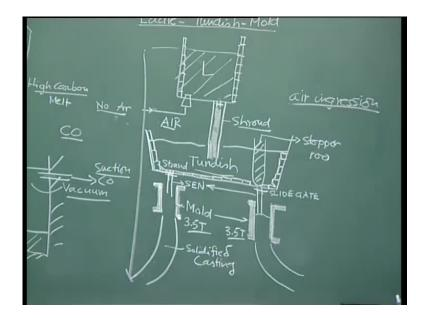
So, for example, in industry, we can see that we can have 3.5 tonnes per minute. That is the rate of casting in a conventional steel plant or steel mill.
