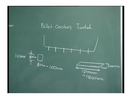
So, therefore, it is understood that if we are talking of a casting rate, that plant demands that we have a casting rate of about through one continuous casting 8 tonnes per minute for example. In that case, it is understood that if you have a billet cast at tundish, if the tundish is producing billet or casting billet, billet casting tundish, you will have more number of strands.
