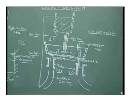
I have drawn a tundish which is a bare tundish. There is nothing inside the tundish. The material is coming from the ladle; it is flowing out. So, that is how the materials goes and flows out of the strand. This is not desirable in tundish as I am going to explain to you. So, therefore, inside of tundish will contains some furnitures and this will also vary from one tundish to another.
