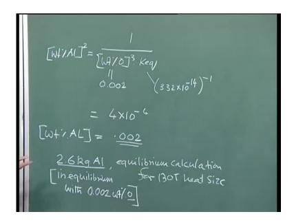
And this is 230 kg of aluminum in equilibrium with 0.002 weight percentage oxygen. So, I come back here; I have already obtained 84 kg approximately; 84 kg to be the thermodynamic stoichiometric requirement on the basis of this calculation. So, this figure weight percentage of aluminum is this much; so, I can translate it very easily that in 100 kg, I have 0.002 kg of aluminum.
