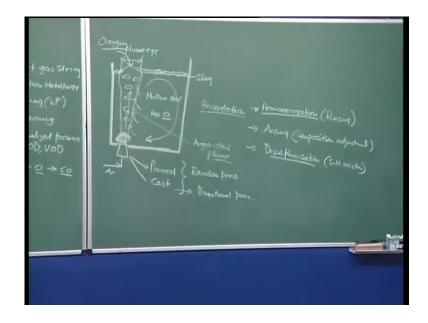
So, argon plus steel, let me give you a clarified picture. Now, having given you the design on the refractory features, let us now draw about it. So, I have the ladle here; I have the porous plug here. I inject argon and what I see is a region here through which bubbles, this is the slag layer. So, this is slag and this is my refractory lined ladle and this is molten metal, molten steel and this is what I am talking about.
