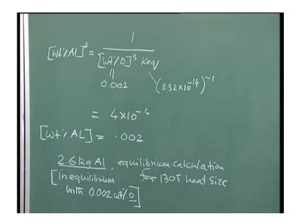
So, if I substitute the value of K equilibrium, what is the final level of oxygen? That is already given to us, which is equal to 0.002, and then, from this particular equation, we should be able to find out that what is weight percentage aluminum, and now, I go to other side, and from this by substituting the value, I can say that weight percentage of aluminum square is going to be equal to 1 inverse 1 by weight percentage of oxygen cube into K equilibrium.
