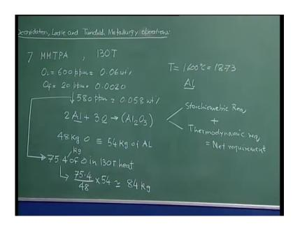
Is to carry out a simple approximate deoxidation calculation, and demonstrate that how one can really calculate the total amount deoxidizer which are needed, let us consider which has an annual production of about 7 million metric tons per annum and let us say that the size of a heat is about 130 tons. So, that implies that the size of the ladle or the vessel we are talking about 130.
