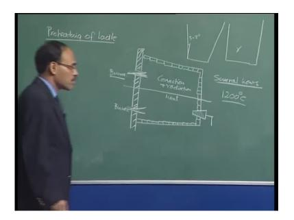
Now, before I proceed further, I would like to talk about little bit about the initial part of ladle pretreatment; that means, when we bring the ladle below the basic oxygen furnace to tap the contents of the furnace into the ladle, the ladle requires to be preheated and the preheating is basically carried out in gas fired furnace preheating of ladle.
