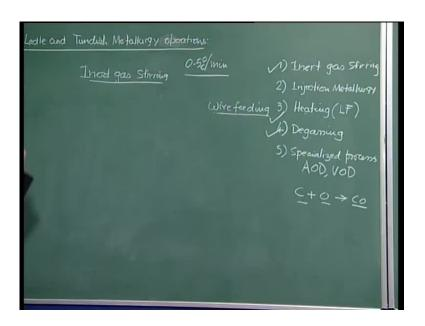
The oxygen injected reacts with carbon produces some heat and also carbon monoxide and this is again vacuum oxygen decarburization, because you have the reaction dissolved oxygen and dissolved carbon, and we know that smaller is the partial pressure of carbon, larger is the tendency of the reaction to go from left to right.
