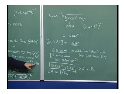
Now, we can sum this to up, and then, tell us that, well, the net requirement is going to be approximately 86.6 kg. So, for every 130 ton heat size, we are going to require. Now, 86.6 kg of aluminum which is to be added, and now, if I translate it to 7 million tonnes of steel, you can imagine that value and it is going to come out to be something like, I think 5,00,000, approx 5,000 tonnes of aluminum.
