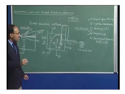
Inert gas stirring that we briefly introduce this terms essentially tells about introduction of argon gas into molten steel. Why we use argon? Because we must understand that we are now continuously refining steel. We are producing; we have removed decarburization. We used crude steel; we have removed oxygen; we are going to take out subsequent operation.
