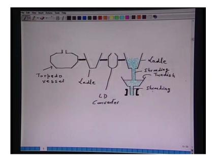
Now, after this, let us see, the iron and steel industry, where the refractories are used. Here I have just shown a schematic sketch of various vessels, where refractory material are used. The first one is a torpedo vessel. Now, this torpedo vessel typically, handles hot metal from blast furnace and transfer it to the LD steel making. That means, this torpedo vessel is the vessel which handles hot metal at around 1300 to 1450 degree Celsius and hence refractory has to be used.
