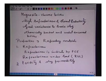
Another example, Magnesite - chrome bricks. Naturally the M g O content of these bricks is greater than the chromite. These refractories, their properties, they have high refractoriness and thermal conductivity. Then, great resistance to basic slag, but in environment, these refractories cannot be used. These refractories are, say chemically bonded and metal encased bricks.
