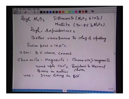
Now, next, for example, high Alumina refractories. Typical example, for example, sillimanite, which contains Al 2O3, 61.0 percent and Mullite, it contains 70 to 85 percent Al 2O3.
