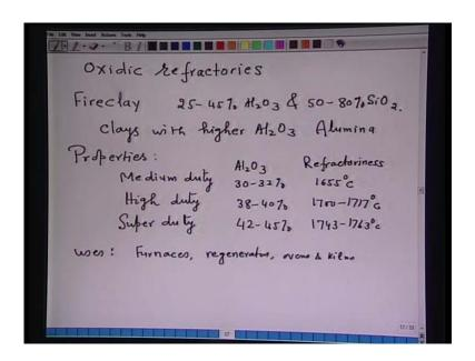
So, continuing with the last lecture, let us take some examples of Oxidic refractories.I will take few examples; for example, the most commonly used refractory is fireclay.Common fireclay contains 25 to 45 percent Al 2O3 and 50 to 80 percent Si O2.Clays with higher Al 2O3 content, with higher Al 2O3 are called Alumina refractories.
