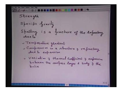
Another important point, is the strength of the refractory. Strength of the refractory - theresistance of the refractory to compressive load, tension and shear stresses. Now, when we design the taller furnaces, then the refractory has to support a heavy load. Hence, strength under the combined effect of temperature and load is important. So, that is the importance of the strength of the refractory.
