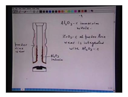
Now, another important that I can show you, this is the immersion nozzle, which is used for continuous casting of molten steel. From the Tundish the liquid steel enters into the mold and this is being done by nozzles and these nozzles are made of Al 2O3- C immersion nozzle. Now, you see, in the mold this particular nozzle is dipped into the mold and the mold is covered by fluxing. So, this area you are seeing here, this is the powder line wear.
