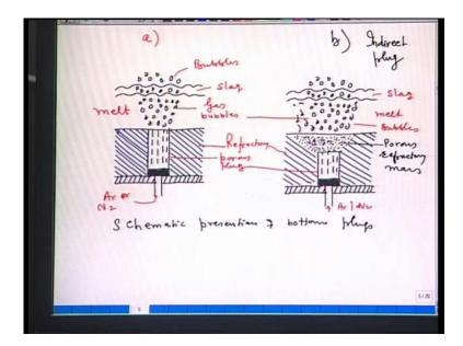
Obviously, advantages of the indirect type of plug is, a large surface area of the bath will be covered. The stirring will be better, but then one has to also design, fabricate and manufacture the porous refractory mass, so that, it allows the gas injection. So, these are the, one of the important differences between the two types of plug. However, there could be another designs also. So, further developments in electric arc furnace will be covered in the next lecture. Thank you.
