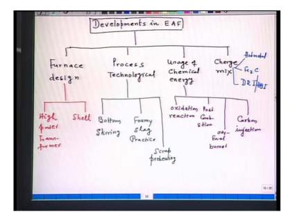
Now, what I am going to do, I will now classify the developments in the electric arc furnace. I will make a diagram for you, the developments in electric arc furnace. So, developments in electric arc furnace has taken place principally, say one, in the furnace design. Another development took place, process, technological process technological
