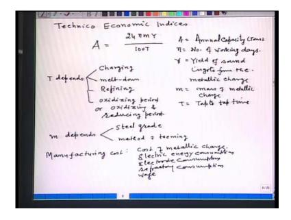
Now, let us see the techno economic indices. Say, A you write that is equal to 24 n m y upon 100 T, where A is annual capacity in tons, n is number of working days and Y, that is yield of sound ingots from the metallic charge, m mass of metallic charge and T is tap to tap time. Now, naturally, if m increases, annual capacity increases, n number of working days increases, capacity increases and above all, tap to tap time decreases, annual capacity also increases.
