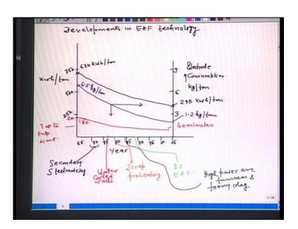
Around 75 this year, water cooled walls were introduced. Water cooled walls, side walls and the roof, they were introduced and that also contributed to decrease in tap to tap time, decrease in power consumption as well as the electrode consumption also. In around 80s, scrap preheating technology was introduced. Preheat this scrap, you are introducing certain amount of energy into the furnace, naturally, the power consumption will also be decreasing.
