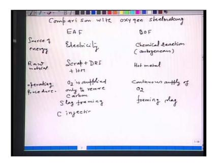
Now, a brief comparison with basic oxygen steel making, comparison with oxygen steel making, say here, I will put electric arc furnace. Here I will put BOF, that is basic oxygen furnace. Now, first differentiation is source of energy. In electric arc furnace, the principle source of energy is electricity, whereas, in basic oxygen furnace, this chemical reactions, they supply the required amount of heat to the process or another way you can call BOF is autogeneous.
