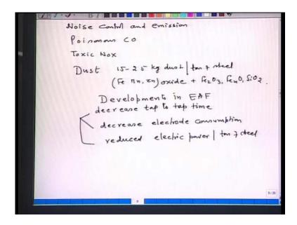
Now, a little bit about noise control and emissions, noise control and emissions. Now, if you happened to see an electric arc furnace plant, that is a mini steel plant, and if you happened to be there during the melt down stage, then you will understand the sound and the noise that is created by the production of the arc, that is, when the electrodes are lowered, a very large amount of sound is being produced because of the arc and so on.
