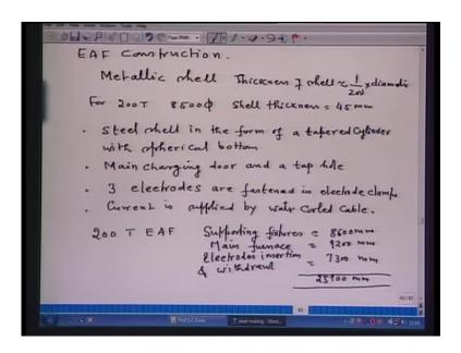
Now, with this, let us go to the electric arc furnace construction. Of course, metallic shell and thickness of shell isapproximately 1 by 200 times diameter of the furnace. So, for example, if we have 200 ton electric furnace, 8500 is the diameter of the shell, then the shell thickness is around 45 millimeter.
