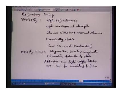
Now, say another important refractory lining, because refractory lining. A metallic shell, it cannot be use for production of the steel. All the heat will be lost. Metal and slag will
