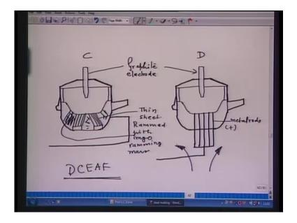
There are two further arrangements are available for fixing of the anode, which is shown in figure C and D.Again in C and D figure, this is the graphite electrode, but, the anode is different in both the cases.In C, the anode consist of thin sheet andthis is rammed with magnesia MgO ramming mass, that means, this is the bottomand this is the so called, ramming mass.
