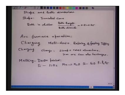
Of the shape and dimensions of bath. Shape of the bath is atruncated cone with a smaller base at the bottom, combined with a spherical segment, as I have said earlier also, it is easier and faster to collect liquid metal pool in the spherical bottom.
