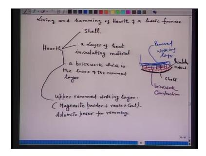
Now, say lining and ramming of lining and ramming of hearth of a basic furnace. Now, here again, I can tell you that, there are acid furnaces or there are basic furnaces. Acid electric arc furnace can be used only for melting purposes, but, in the basicEAF, one can do refining also. The main difference between the two is in the refractory lining.
