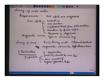
Then, let us see lining of sidewalls. Now, the shell is first covered with asbestos sheet, fireclay bricks ((being then)) and then rammed with the working layer. Same as what you have done for the hearth, first the shell will have the asbestos sheet, for insulation purposes, followed by the fireclay and followed by the ramming mass, because that, that ramming mass will be in contact with the slag metal and gases.
