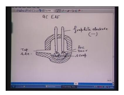
In alternative current electric arc furnace, the combination of electrode and cathode that looks as shown in the figure. So, this is a graphite electrode, which is negatively charged and this is, the scrap, which also acts as an anode. This is the arc, which is produced when graphite electrode hits the scrap. This is the door or charging. This is the tap hole. So, that is how the arrangement of electrode looks in AC EAF.
