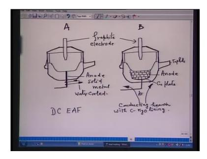
Now, another combination of electrode is DC electric arc furnace, which is shown in figure A and B.Now, in figure A and B, this is again the graphite electrode, this also a graphite electrode.
