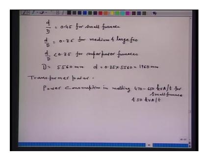
So, a ratio between the pit circle diameter, the electrode and diameter of the bath is of the order of magnitude, which I am giving you here, if d is the pit circle diameter of the electrode, where all the 3 electrodes are arranged at the apex of an equilateral triangle and D is the bath diameter, then this is approximately equal to 0.45 for small furnaces, d by Dis equal to 0.35 for medium and large furnaces and d by D less than 0.35 is preferred for super power furnaces.
