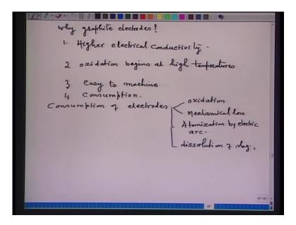
Now, why graphite electrodes are preferred than carbon electrodes? Because, graphite electrodes have higher electrical conductivity. Higher electrical conductivity means higher current density is possible and lower electric losses will be there. Ultimately, you will be supplying electricity and the losses are more, well, you have to supply more amount of electricity.
