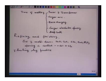
Now, the time of melting, it depends on the following factors, it depends, first of all, on power of the transformer, power of transformer.
