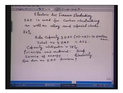
Mini steel plants have contributed to the growth of electric furnace steel immensely. Presently, electric arc furnace is used for carbon steel, for carbon steel making as well as alloy and special steel. Electric arc furnace is used for production of long products, but, nowadays, flat products are also being produced.
