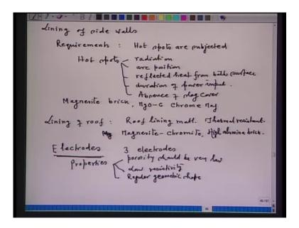
So, the roof lining material, as such, should be thermal resistant. So, roof lining material should be thermal resistant. That is, one of the very important property. Preferred roof material, they are Magnesite, Chromite or high alumina brick.
