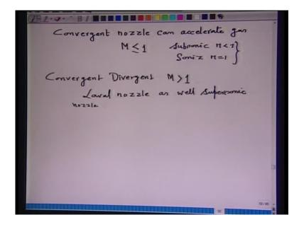
So, convergent nozzle can accelerate gas from some velocity to maximum up to M less than or equal to 1.So, these type of nozzles are called subsonic, when M is less than 1 and sonic, when M is equal to 1.So, such nozzles are called subsonic to sonic nozzle, depending on the value of Mach number at the exit of the nozzle.
