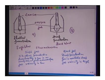
And, one with 0.46 meter which is called a deep penetration of the jet.And this shallow and deep, I have shownin this particular figure, where you note that, this is a sort of a profile of a converter, this is the lance, this is the oxygen jet.So, in one case, the distance between the bath and the lance is greater, in a, in b, the distance between the bath and the lance is lower.
