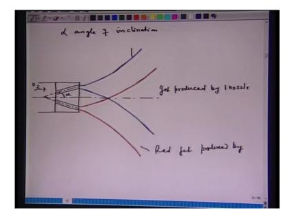
So, in this figure I have shown that, how the angle of inclination affects the jet coalescence. In this particular figure, the flow rate of oxygen is coming in this direction and this is, the blue one is the jet produced by 1 nozzle and red one is jet produced by another nozzle.
