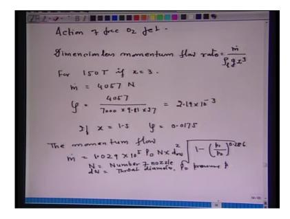
Now, as I have said, it is difficult to find out the velocity, but, we know that mass of the jet increases downstream the distance. Velocity of the jet decreases. So, the momentum of the jet, that is, m into v is conserved downstream the nozzle. That means, the momentum flow rate within the jet is constant and that is a very important property.
