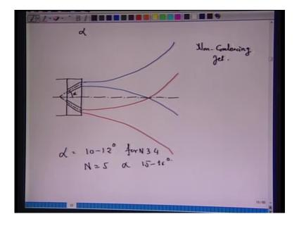
In this figure, what I have done, I taken alpha as, such that, the jet issued from each nozzle, they coalesce at a higher distance downstream the nozzle.
