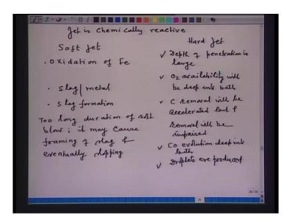
So, for example, if the jet is chemically reactive, then, what this soft jet and hard jet means? A chemically reactive jet means, again the jet has mass and velocity. So, mass of
