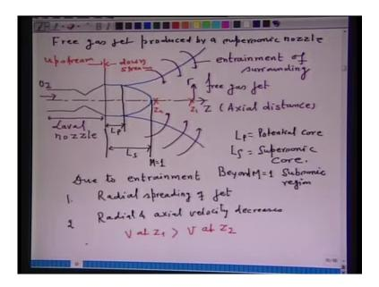
Now, a gas exiting the nozzle spreads in the surrounding and is called a free gas jet, as shown in this particular figure. So, this is a free gas jet produced by a supersonic nozzle. So, this portion is the free gas jet. You see that, the jet begins to be spread as the gas exits the nozzle. Now, this particular portion is the Laval nozzle. This is the direction of flow of, for example, oxygen.
