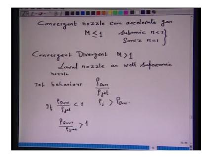
So, in fact, the jet behavior, it depends upon the density ratio or that means, density of surrounding upon density of jet.A ratio equal to 1, the density of jet is that of surrounding.So, it is with that reference, I am now comparing a ratio, when it is less than 1 or when it is greater than 1.
