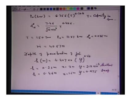
Here N is the number of nozzle, d N is the throat diameter,P0 is the pressure, supply pressure rather, and p is the atmospheric pressure.Now, this pressure P0, it can be calculated by P0 in bar, that will be equal to 6.755T raised to the power 0.104, where T, that is equal to capacity in tons.
