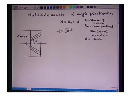
This is the angle of inclination, alpha is the angle of inclination of each nozzle with the excess of the lance. This is the lance, is the excess of the lance and alpha is the angle of inclination. Now, this angle of inclination will decide whether the jet produced by independent nozzle will coalesce downstream the nozzle or will not coalesce downstream the nozzle.
