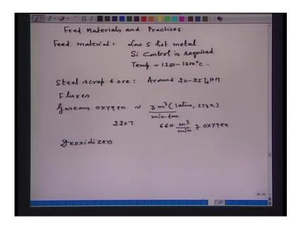
So, let us take now the feed materials and practices. Now, feed material say, one requirement is low sulphur hot metal. Why low sulphur hot metal, because in steel making, sulphur removal is not possible. Then silicon control is also required. For larger is
