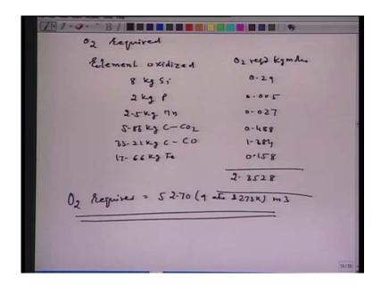
Now, we can calculate now the amount of oxygen required the oxygen required silicon to Si O 2 carbon to CO 2 carbon to CO M n to M n O and all these oxidation reactions they are to be written and accordingly you find out the amount of oxygen that is required how much amount of element is being oxidized. So, if I write immediately say element oxidized and then oxygen required in kg moles.
