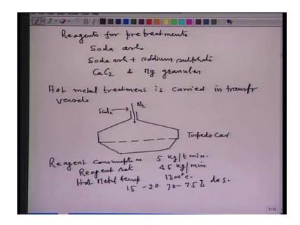
Now, the reagents for pretreatment soda ash then soda ash plus sodium sulphate calcium carbide and magnesium granules now for your information magnesium is a very strong desulphurizer. Now, this reagents can be added or they can be injected now hot metal pretreatment is done is carried out in transfer vessels now you know that when hot metal is carried over to 1 d shop then it is carried over in a torpedo ladle.
