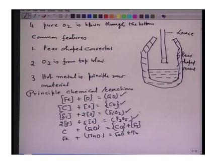
Now, this particular which is called bottom blowing steelmaking is hardly used any in any part of the world it is just a modified version of basic bessemer process where air was injected in 1878 instead of air in the modification oxygen was introduced through the bottom, but, as a bottom blowing steelmaking pure bottom blowing steelmaking is not practiced to my knowledge.
