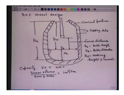
Now, let us go to the B O F vessel design now typically B O F vessel it look something this way this one. This is a refractory lined vessel this is this height is called H b this dimension is diameter of the path this is the top lance fitted with nozzles and this distance from here to the metal height is called lance distance.
