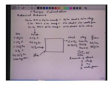
Now, let me go to the charge calculation. In fact, for charge calculation one has to do material balance and material balance input must be equal to output.
