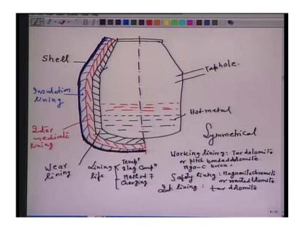
Now as regard the refractory lining that is shown in this particular figure the outside one you have the shell and first you have the insulation lining which is backed by the intermediate lining and then you have the wear lining.
