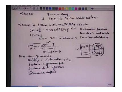
Now, let us see the lance .Lance in fact, is a heart of converting steelmaking it is 8 to 10 meter long the diameter of the lance is varies from 20 centimeter to as high as 25 centimeter and it is water cooled it is water cooled. Water cooling at the rate of 50 to 70 meter cube per hour at 5 or to 6 kilogram per centimeter square pressure the lance is fitted with multi-hole nozzles.
