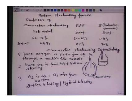
Now, modern steelmaking practice it comprises of say converter steelmaking then electric arc furnace steelmaking and small portion of a steel is also made in the so, called IF that is the induction furnaces I will put it induction furnaces.
