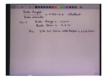
That means the capacity of the converter increased by increasing the diameter rather than the height because if you increasing the height then the shop becomes very tall because you have to charge everything from the top. So, the capacity of the converter is increased by increasing the diameter of the bath rather than the height.
