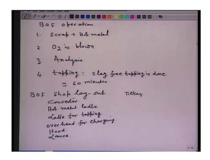
So, B O F operation it first of all consists of a scrap plus hot metal, that means, we charge scrap top operative charge hot metal, but, the principle feet is the hot metal which is 60 to 70 percent depending on the heat balance and rest could be scrap takes around two to three minutes for charging.
