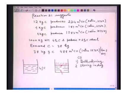
Now, for example, again I take a steel bath. It is hot metal, containing four percent carbon. I am providing oxygen. There is no clay cover in the beginning, then whatever the amount of CO which is evolving due to oxidation of carbon will be exiting uninterruptedly and continuously from the bath, because there is no hindrance. So, that is one extreme.
