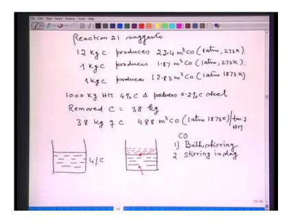
So, now this reaction 21 suggest, what it suggests, say 12 kg carbon produces 22.4 meter cubed carbon mono oxide at 1 atmospheric pressure and 273 Kelvin.
