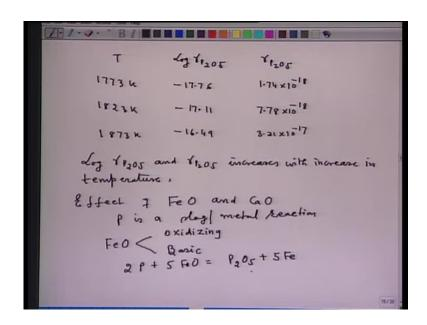
So, for example, I take here temperature, I take here log gamma P 2 O 5 and I calculate here gamma P 2 O 5. I take 3 temperatures 1773 Kelvin, 1823 Kelvin and 1873 Kelvin. I calculate log gamma P 2 O 5 minus 17.76, minus 17.11, minus 16.49, gamma P 2 O 5 is 1.74 into 10 to the power minus 18, and 78 into 10 to the power minus 18 and 3.21 into 10 to the power minus 17. Now, what is the conclusion?
