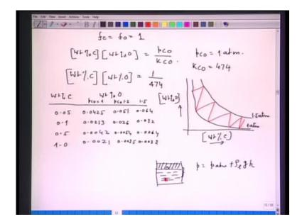
So, accordingly I will write down p CO, f C into weight percent carbon, f O weight percent oxygen and let us call this equation as 22. Now, assuming, the activity coefficient of carbon and oxygen in liquid steel to be unity, however, this value may not be unity, but, for the sake of calculation and understanding, let us take that f C is equal to f O, that is equal to 1.
