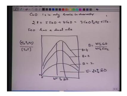
Now, as regards calcium oxide, calcium oxide cannot provide oxygen for reaction with phosphorous. So, calcium oxide, it is only basic in character. Now, from the definition of
