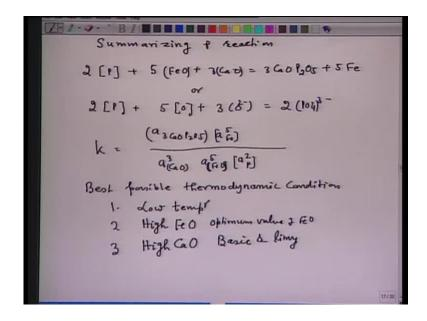
So, in fact this optimum Fe O, this optimum Fe O is around 15 to 20 percent of Fe O. So, that is what about the effect of Fe O and Ca O. Now, summarizing this, now, summarizing the phosphorous reaction, you can write down 2 P plus 5 Fe O plus 3 Ca O, that is equal to 3 Ca O P 2 O 5 plus 5 iron or in the ionic form, we can also put it, 2 P plus 5 O plus 3 O 2 minus that is equal to 2 P O 4 3 minus.
