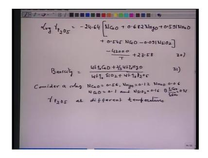
Log gamma P 2 O 5, that is equal to minus 24.64 N Ca O plus 0.682 N MgO plus 0.591 N MnO plus 0.545 N Fe O minus 0.091 N SiO 2 minus 42000 T, now here the T is in Kelvin, plus 23.58 and this is equation number 30.
