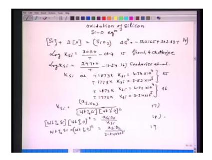
So, next reaction is oxidation of silicon. In fact, we are considering silicon oxygen equilibrium. So, if I write the reaction, silicon plus 2 O, that is equal to Si O 2. This rounded brackets, I am using for slag, and square bracket, I am using for dissolved in metal. Delta G naught, the value is minus 542165 plus 202.83T. Now, this is equation number 14.
