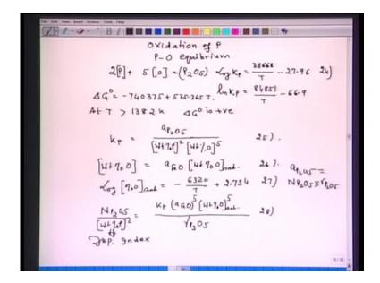
So, let us consider the next reaction, oxidation of phosphorous, or phosphorous oxygen equilibrium. That is 2 P in metal plus 5 O that is equal to P 2 O 5 in slag. Log of K P, that is equal to T minus 27.96. This is called equation number 24. Now, again I could get another source also, which says this l n K P, that is equal to 84851 upon T minus 66.9.
