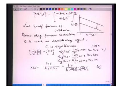
So, we write down now, weight percent oxygen, that is equal to 0.308 into 10 to the power minus 5 upon weight percent silicon raised to the power 1 by half.
