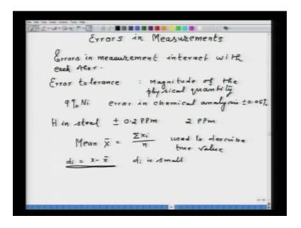
In fact, the errors in measurement interact with each other. Now, here, one should also be clear that something like error tolerance. Now, this error tolerance means, how much amount of error you can tolerate in the measurement of a physical quantity. Now, this error tolerance depends upon the magnitude of physical quantity.
