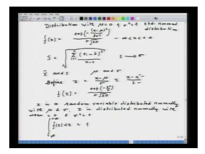
Now, distribution with mu is equal to 0 and sigma square is equal to 1. It is called as standard normal distribution. It can be represented by f x equal to exponential minus x minus mu upon whole square upon 2 sigma square upon sigma into square root of 2 pi and this is valid for minus infinity less than x less than plus infinity.
