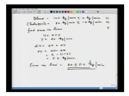
Now, let us take the example of blend and lime stone in chalcopyrite. So, it consist of 100 kg per minute with an error plus or minus 4 kg per minute In our equation, let us call u and say chalcopyrite is 80 kg per minute and with plus or minus error of 1.6 kg per minute. Let us say this as x, find error in lime and call this as y. Then we have u equal to x plus y. We get y is equal to 20 kg per minute. Of course, it is 100 minus 80 kg per minute.
