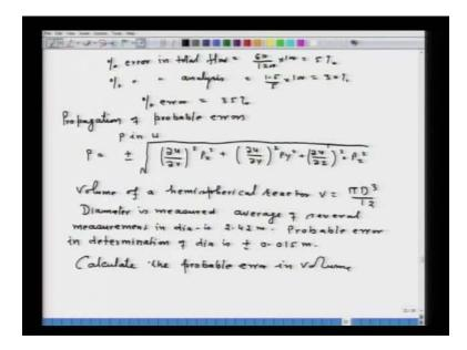
For example, percent error in total flow is equal to 60, then 1200 into 100 is equal to 5 percent. Percent error in analysis is 1.5 upon 5 into 100 and that is 30 percent. So, total error is become 30 plus 5. So, percent error in oxygen flow is again 35 percent, so, in this way also you can do it.
