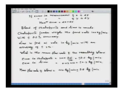
If error in measurement of x is delta x and error in measurement of y error is delta y, then maximum error will be equal to delta x plus delta y. Now, let me illustrate by taking a particular problem. For example, in copper extraction, you roast the chalcopyrite concentrate and you prepare a blend of chalcopyrite and lime. So, a blend of chalcopyrite and lime is made by weighing chalcopyrite and lime independently and then they are mixed into a container and fed into the plant.
