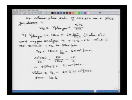
So, let me illustrate this by an example. Now, let the volume flow rate of oxygen in a flue gas stream is equal to VO2 and that is equal to V flue gas into percent O2 upon 100. It is a volume flow rate in oxygen in flew gas and this one gives it (Refer Slide Time: 37:16).
