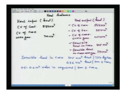
So, let us do the heat balance typically: heat input in kilo calorie, Cv of Coal, and then we have Cv of coke oven gas. Because you are combusting it, Cv of Coal is 8184 in to 10 to the power 3 and that is 704 and 10 to the power 3 here (Refer Slide Time: 15:23).
