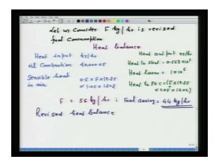
So, let us consider now, F kg per hour is our revised fuel consumption. Now, we can do heat balance. Let us see what heat balance gives us. We can do heat balance. For the heat balance, we take one heat input and heat input is say oil combustion; that will be in kilojoule per hour.
