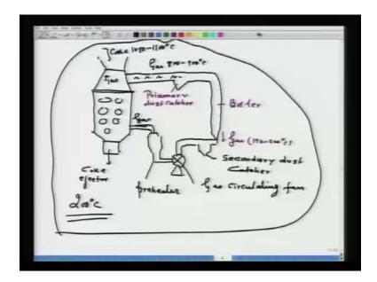
Now, I will just give you a flow diagram of a technology which works on the dry quenching. So, here what do you have? You have a reactor; for example, this is a reactor.
