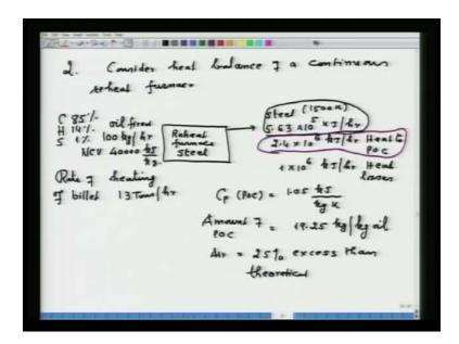
So, I will create a different problem, say on second case. Now, consider heat balance. Consider heat balance of a continuous reheat furnace. I will not be going into detail of all calculations; you can do yourself, what I am representing.
