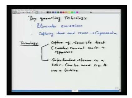
In fact that idea is working in the plant; why not to evolve a mechanism of quenching of coke not by water, but by gas? This mechanism is called dry quenching technology.
