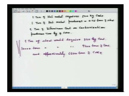
Now, just to give you a figure, say one ton of hot metal, hot metal means the pig iron - it requires 500 kg of coke, approximately. The figure may vary, but just I am taking an example.
