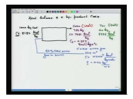
Let us consider the heat balance of a by-product coke oven. Now, here I have selected the heat balance; basically this material balance - first we have to do it. In the lecture 27 which is material balance in coke making, one of the examples which I presented over there, I have used the data of material balance to illustrate the energy balance or heat balance over here.
