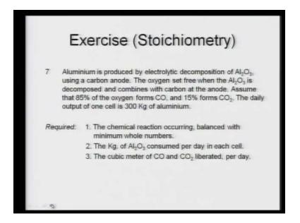
Problem 7: Aluminium is produce by electrolytic decomposition of  $Al_2O_3$ ; it is a very standard and common method for production of aluminum from bauxite. What is being done? From bauxite, first of all  $Al_2O_3$  is brought into solution by leaching; and then  $Al_2O_3$  is electrolyzed as such, because  $Al_2O_3$  has a very high melting point; so, in order to make an electrolyte, you try to dissolve in cryolite; and in cryolite,  $Al_2O_3$  is soluble.
