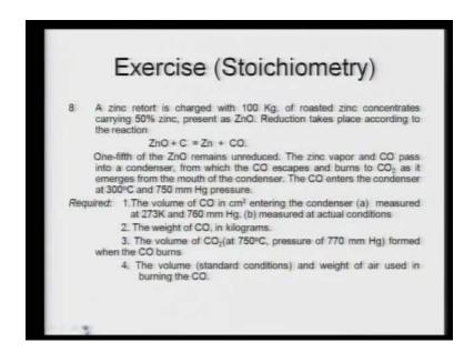
Problem number 8: it is the reduction of zinc oxide by carbon; a zinc retort is charged with 100 kg of roasted zinc concentrate carrying 50 percent zinc, present as ZnO. The reduction equation is given. Now, the problems says that one-fifth of the ZnO is unreduced.
